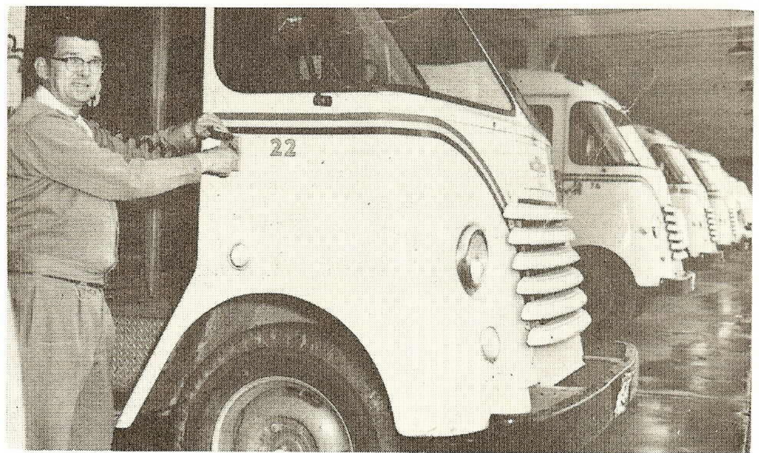
Rainbo salesman Carl Sheffield, plugs in the 220 volt circuit to power the electric heater in his truck. These heaters keep the inside temperature a constant 85° Fahrenheit while trucks are at the loading ramp. Deliveries are made inside Texas in an 80 mile-radius of Beaumont. One delivery is made Monday through Friday and two trips are made on Saturday.
