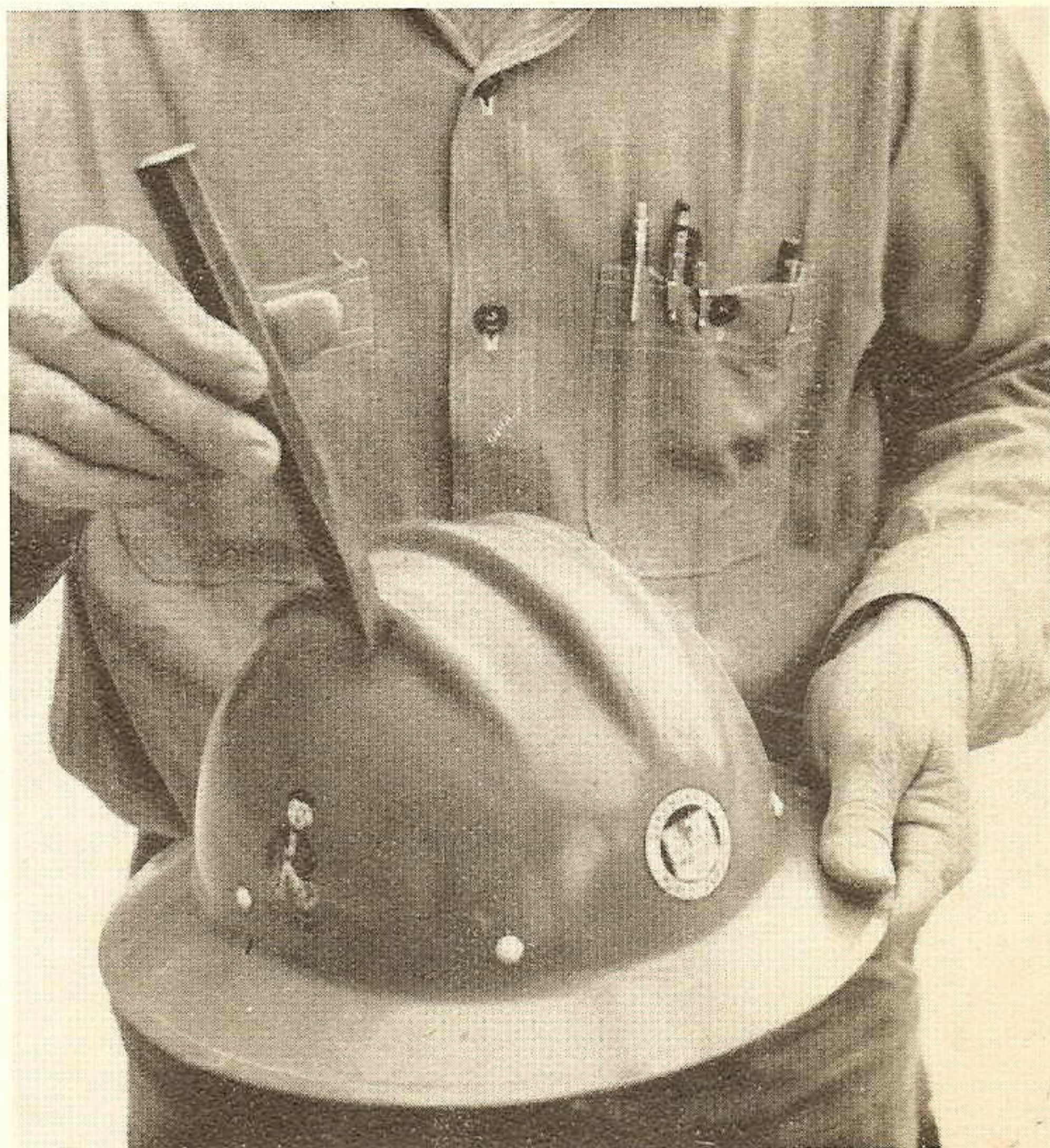
This is where it went. Mr. Hensley shows how the chisel struck his safety hat, after falling 53 feet from #17 boiler.
