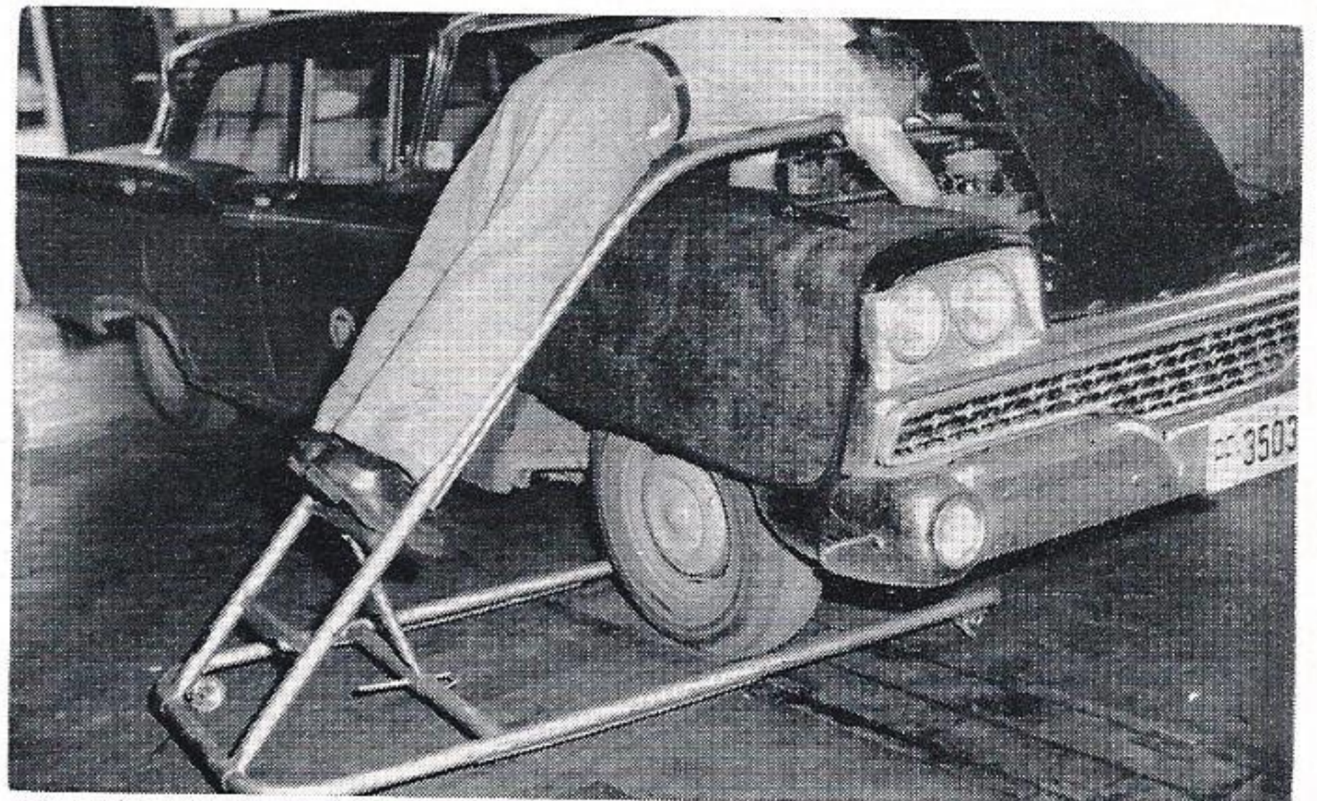
MECHANIC'S PLATFORM —Mechanics work in close quarters on trucks. They needed some way to do the job without straining or mounting an unsafe platform. This apparatus solved the problem. Using it, the repairman can safely and comfortably get to inaccessible places in and around engine areas.
