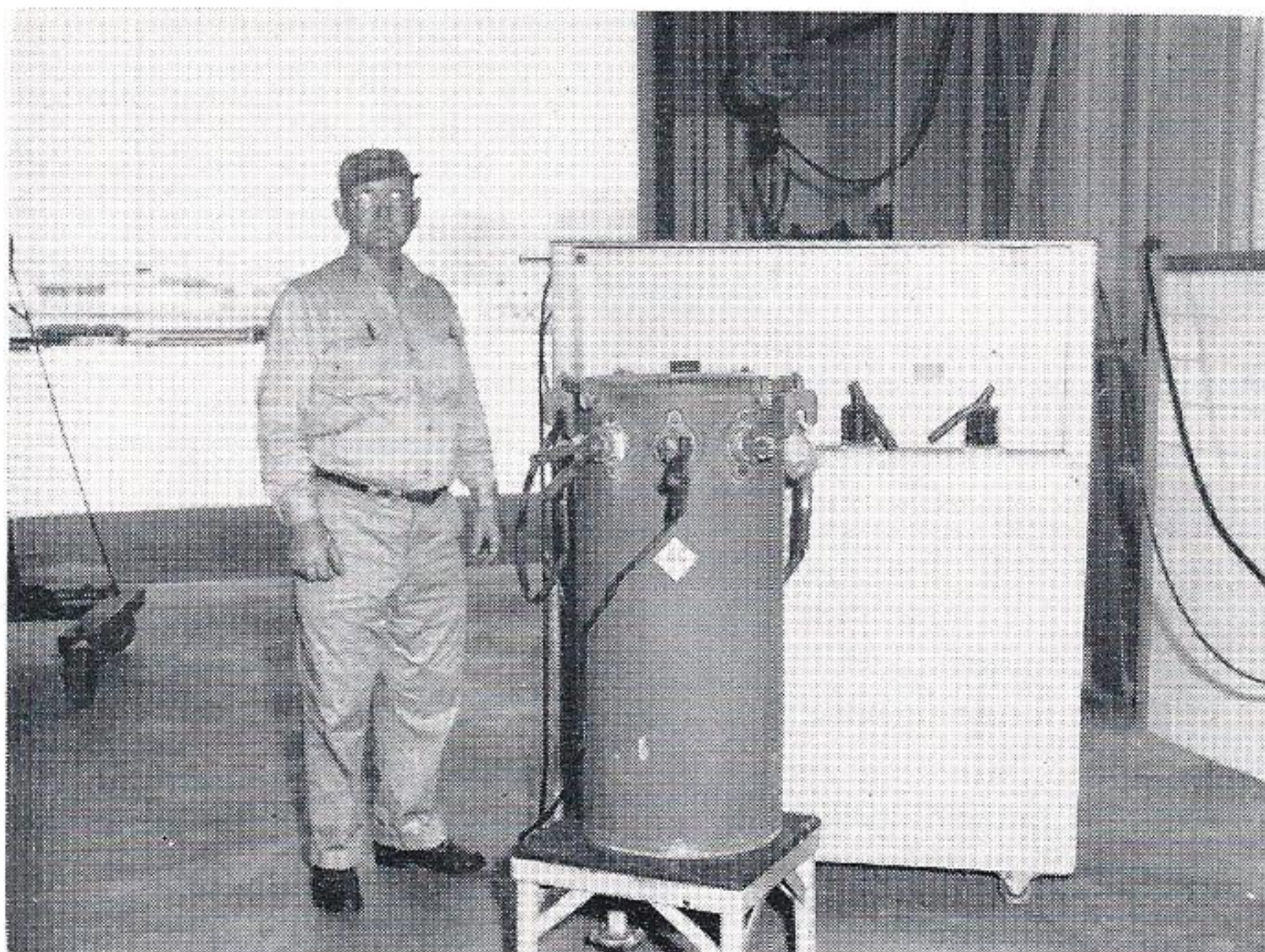
Keeping distribution voltages up to par in neighborhoods throughout the system are the jobs of hundreds of transformers. But the transformers need regular check-ups to stay healthy. R. D. McMillian shows where the power goes round-and-'round to come out these leads and into the transformer to be tested.
