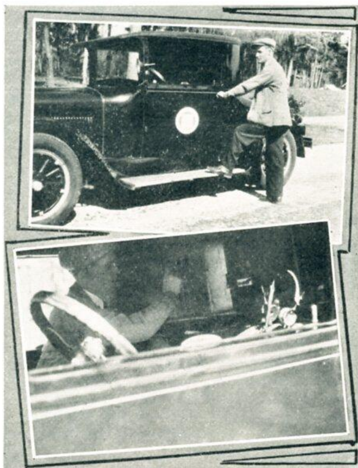
Top—C. R. Nantz on the trail of some radio interference. Bottom—Superheterodyne equipment used in locating interference.
