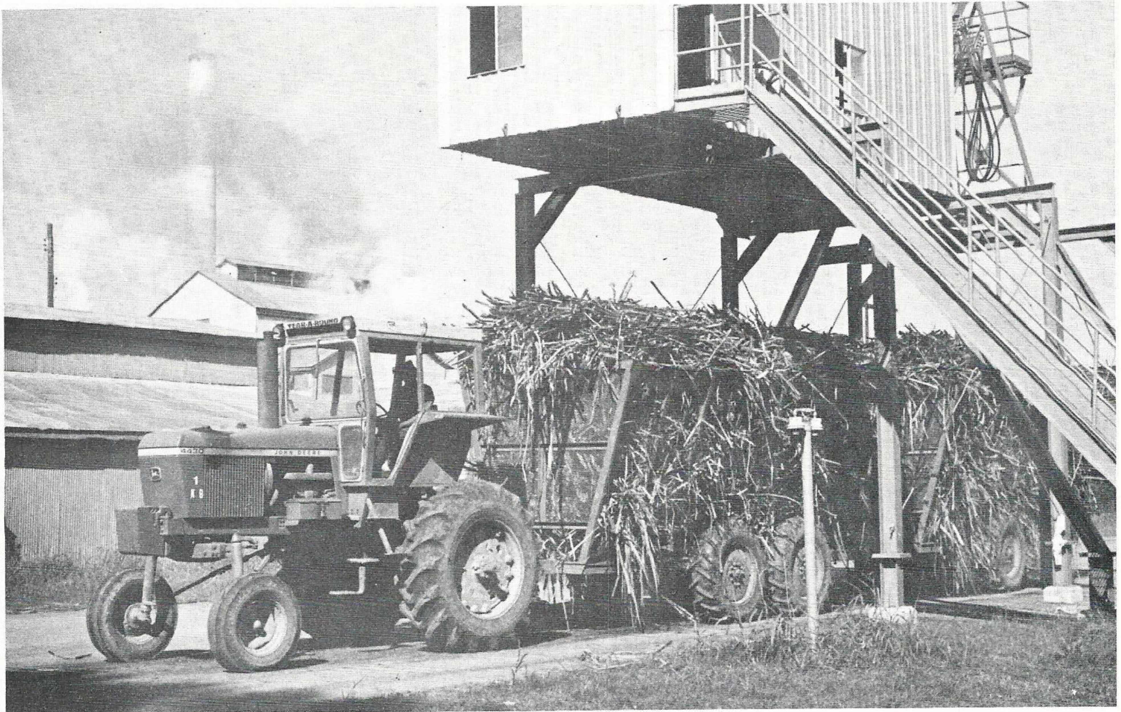
CORE SAMPLER —The St. Martin Sugar Co-operative was the first sugar house in the state to utilize the core sampler. The sampler removes a small portion of each farmer's crop. This cane is then graded in an on-the-grounds laboratory to determine the quality (sugar content) of the cane prior to processing.
