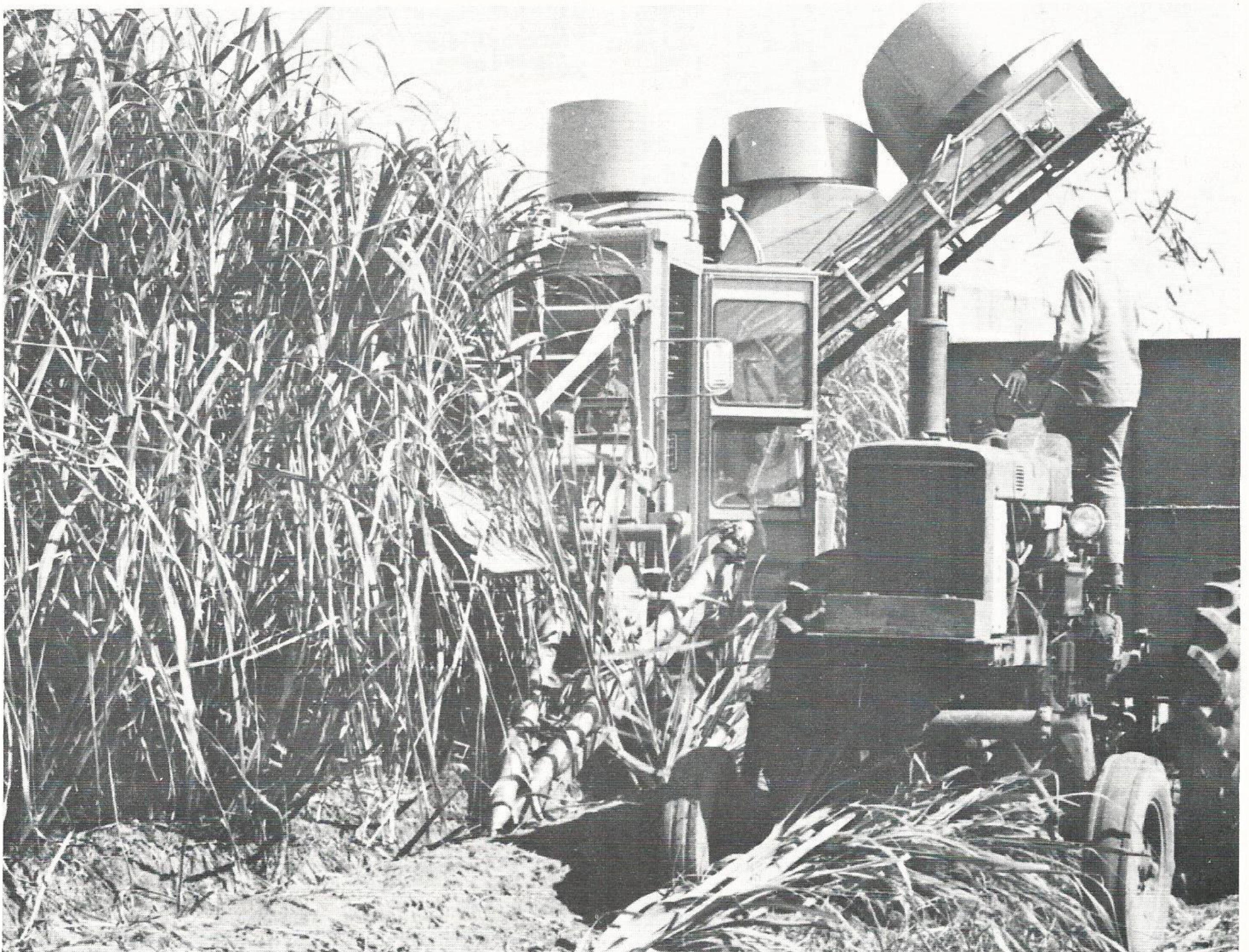
CARY CANE HARVESTER—This Proto-type sugar cane harvester, built by J. C. Cary of Opelousas, undergoes testing by the Co-op. It is designed to harvest some 20 tons of green cane per hour.
