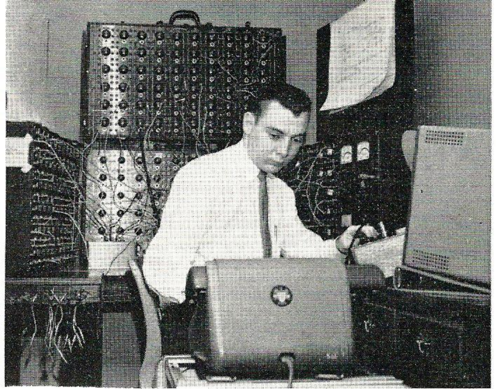
STUDIES "REDDY'S HABITS. The author, Don Lyle, engineering assistant in the Relay Department, Beaumont, runs through a study on the time saving A.C. Network Analyzer recently installed.
