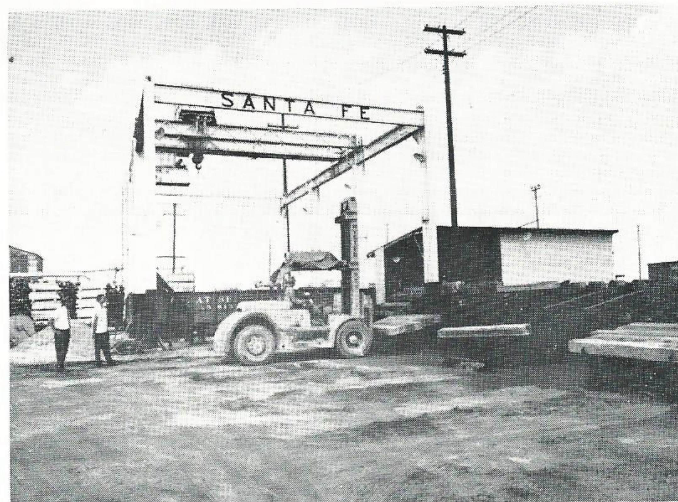
TIMBERS GRADED AND SEPARATED. Mr. Houston, left, and Mr. Stout inspect the unloading, grading and separation of timbers that have just arrived from a sawmill. Timbers are unloaded by an electrically powered overhead crane from rail cars and are separated according to length and type of wood.
