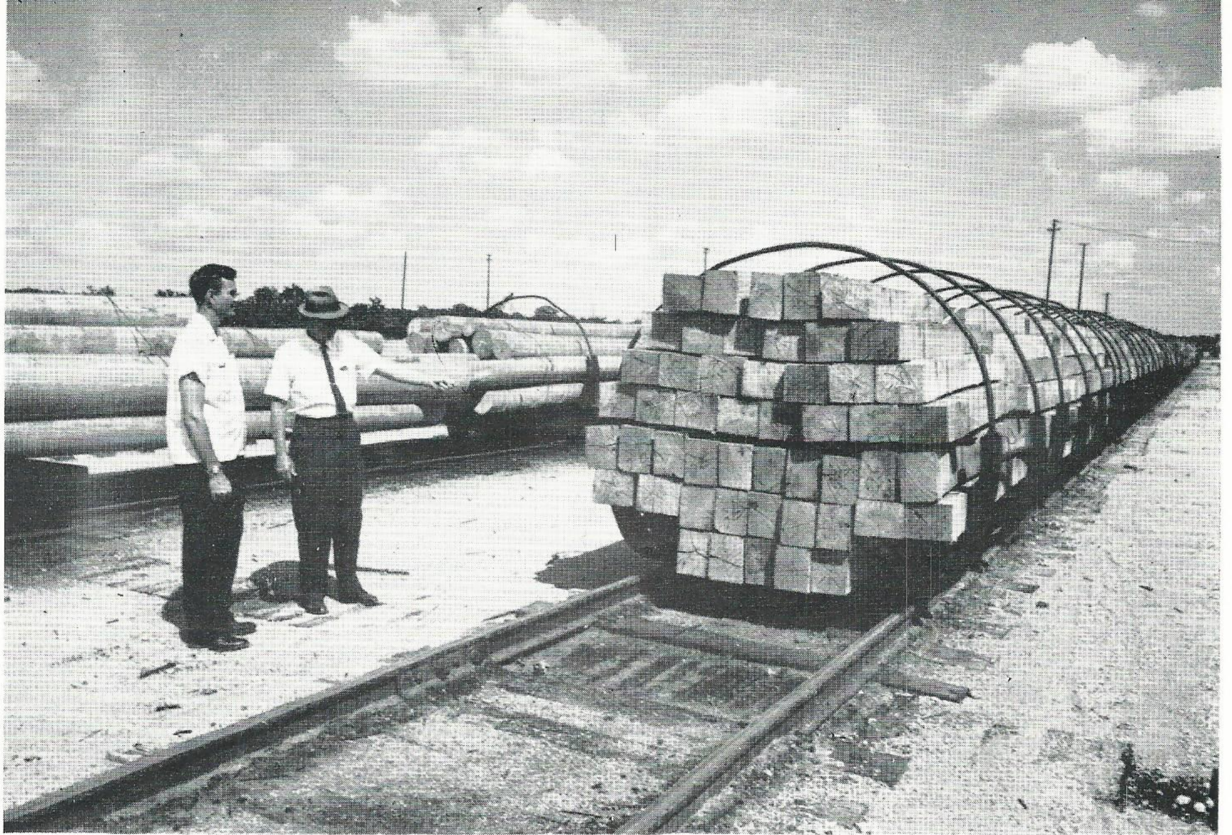
EXPLAINS TREATMENT PROCESS. Mr. Houston explains the construction of rail cars used in the treatment cylinders and the method of process-
