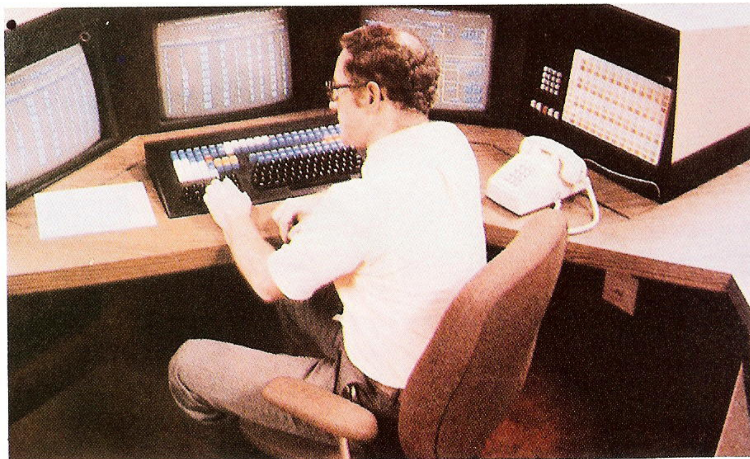
System operators, using a multiple interactive crt console similar to this arrangement, will economically dispatch power throughout the GSU system.
