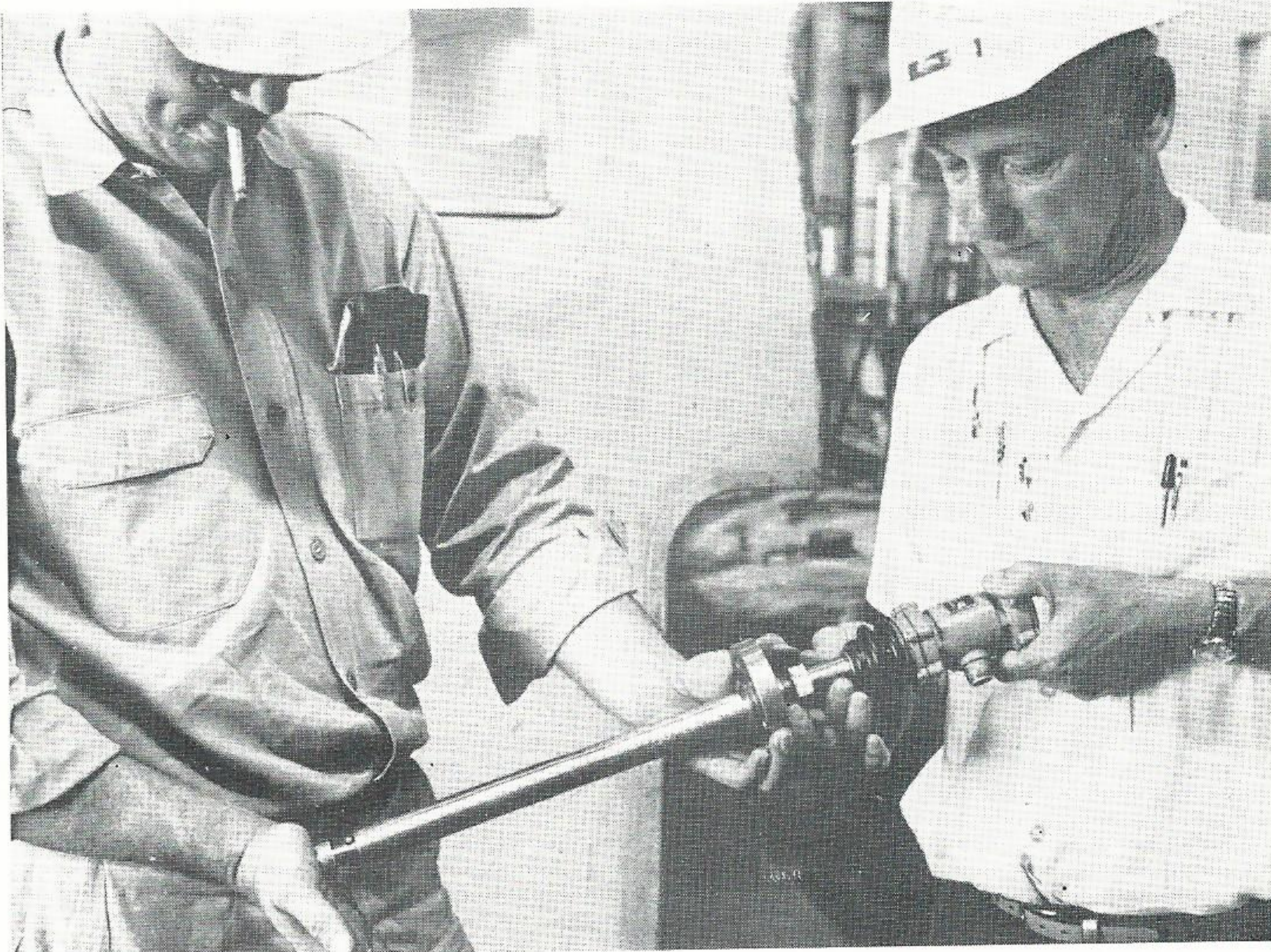
VIBRATION DETECTOR. Mr. Foreman, A-C's construction supervisor, and George Brill, test supervisor, demonstrate a vibration detector which will be added to the turbine spindle.
