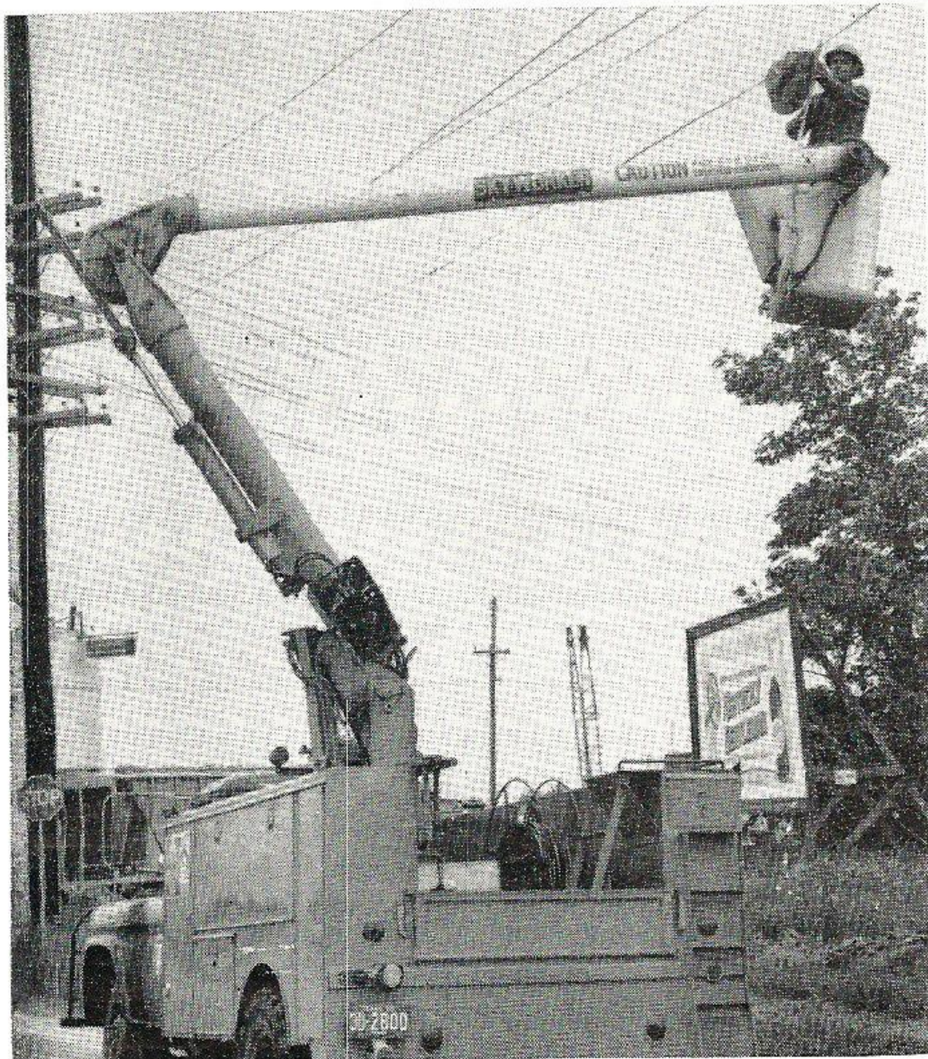
Mr. Beard removes one of the numerous kites that become entangled in the Company's lines each year. The Skyworker's agile maneuverability makes short work of such chores.
