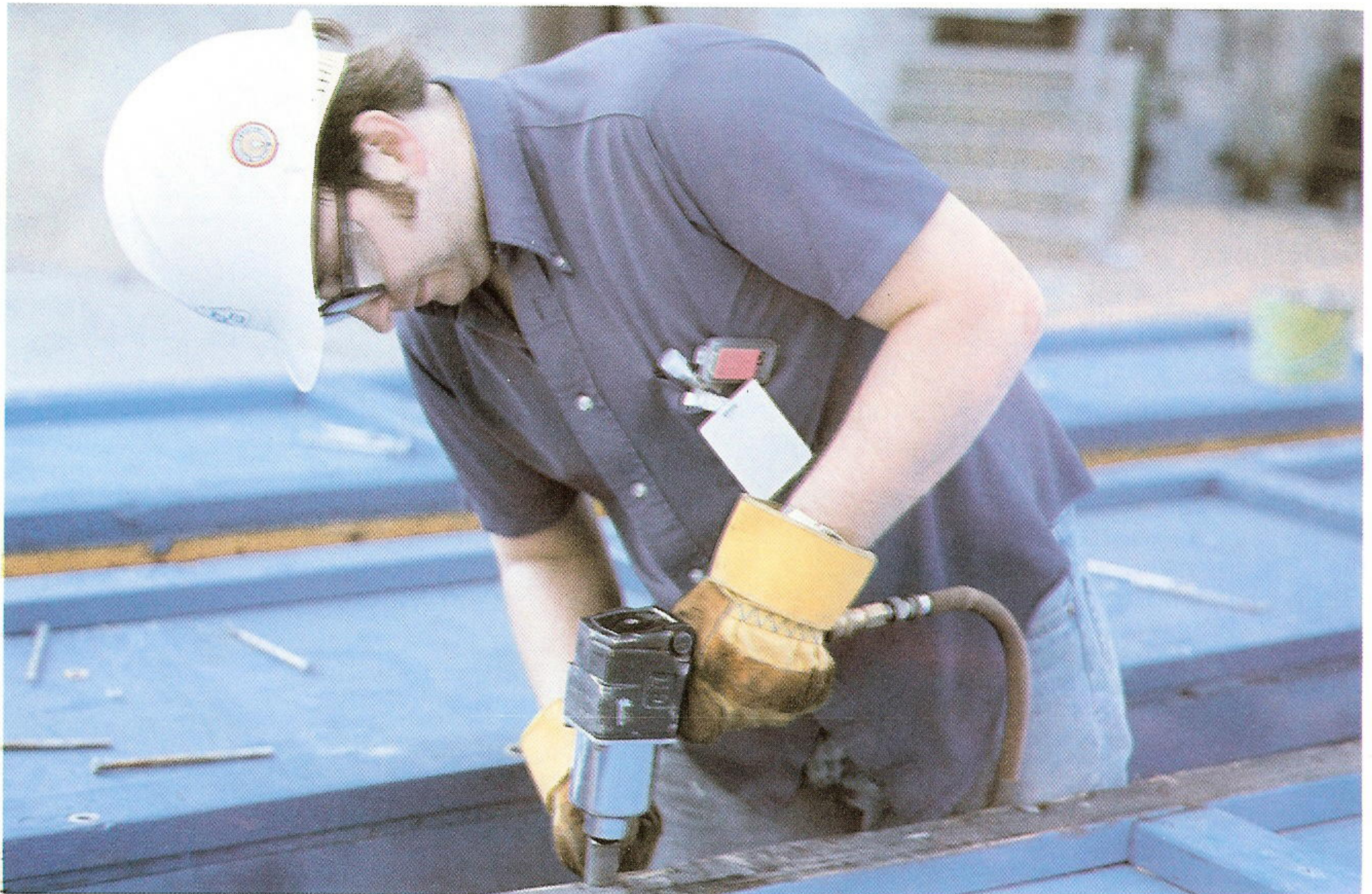
Joe Ison, repairman-1st class-nuclear, removes bolts from a box of fuel bundles.
