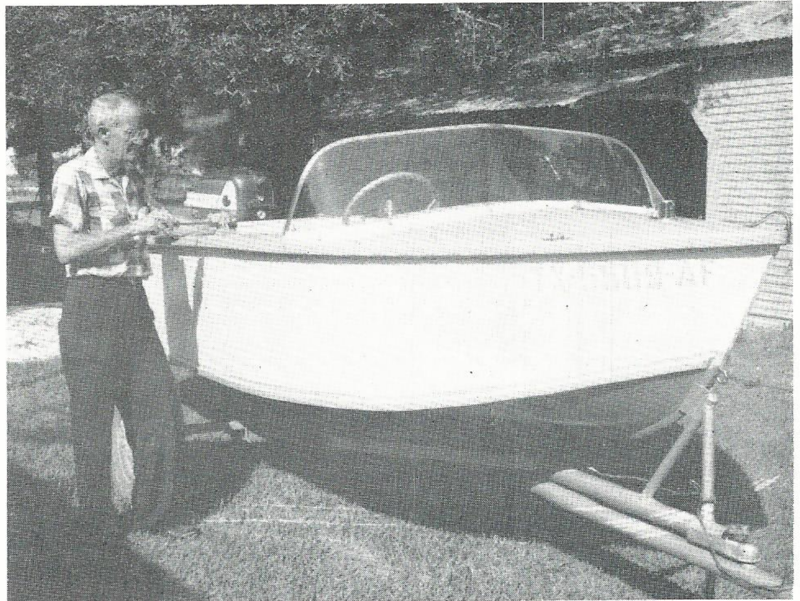
THE BOAT "HAP" BUILT. A. D. "Hap" McMillian, general line foreman, Port Arthur, puts the finishing touches on his new boat. It took "Hap" about two months work in his spare time to build this boat. It is 13½ feet long, 63 inches wide across the bottom and 73 inches wide across the top. The boat is powered by an Evinrude 35 horsepower motor and will carry three passengers. "How fast it will go nobody knows," said "Hap". "It just flies." "Hap" has been using the boat to catch up on his shrimp supply which he lost during hurricane Carla.
