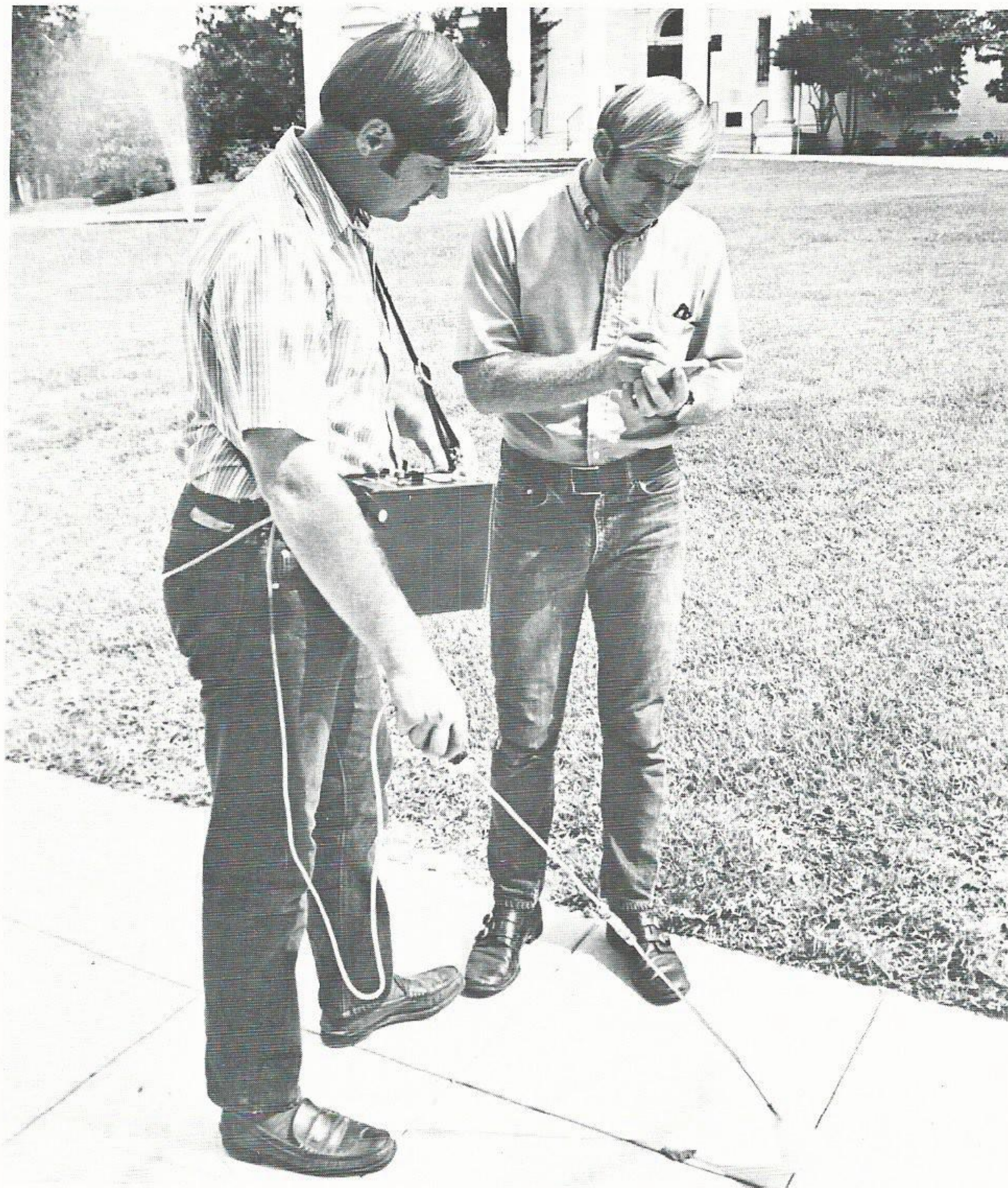
Richard Hebert, left, and James Curtis (Baton Rouge Gas Department) are not hunting for uranium, but for possible gas leaks. These two men are testing a new, super-sensitive device designed to smell out any gas leaks hidden under the ground, even under concrete. The machine is being tested in downtown Baton Rouge, and has caused many passers-by to stop and watch.
