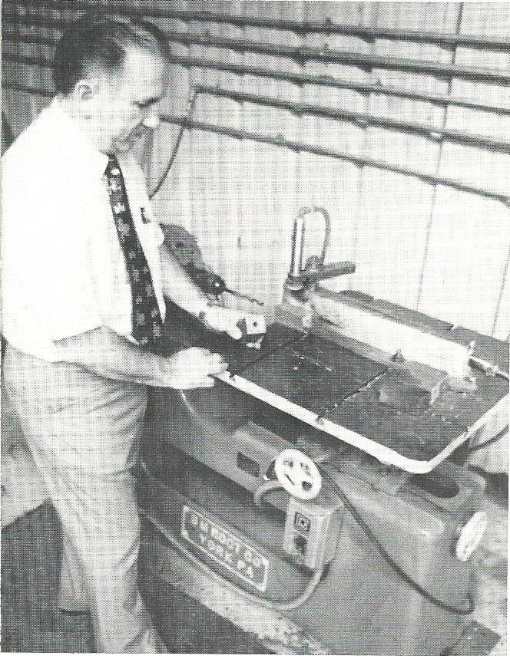
A boring press that can drill 12 calls a minute is one of the early steps in the manufacturing process.
