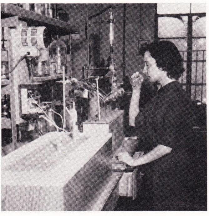
Lab controls check process before, during and after refining, with chemist Wales Newby in charge. Here Mrs. Marlin Brown sniffs oil sample taken from electrical test which determines stability of product. The object is to make sure the oil will keep as long as possible without developing an odor.
