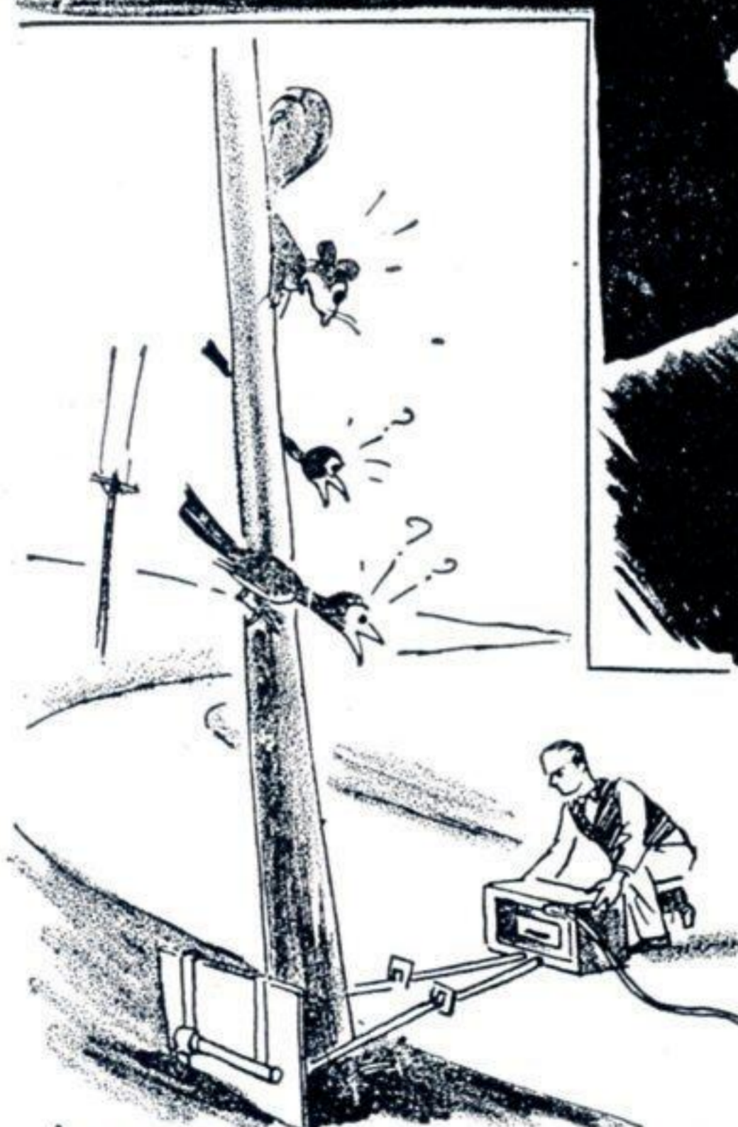
PORTABLE X-RAY MACHINES ARE MAINTAINED BY MANY POWER COMPANIES TO LOOK THROUGH POWER POLES AND DETECT DECAY . . . . .
