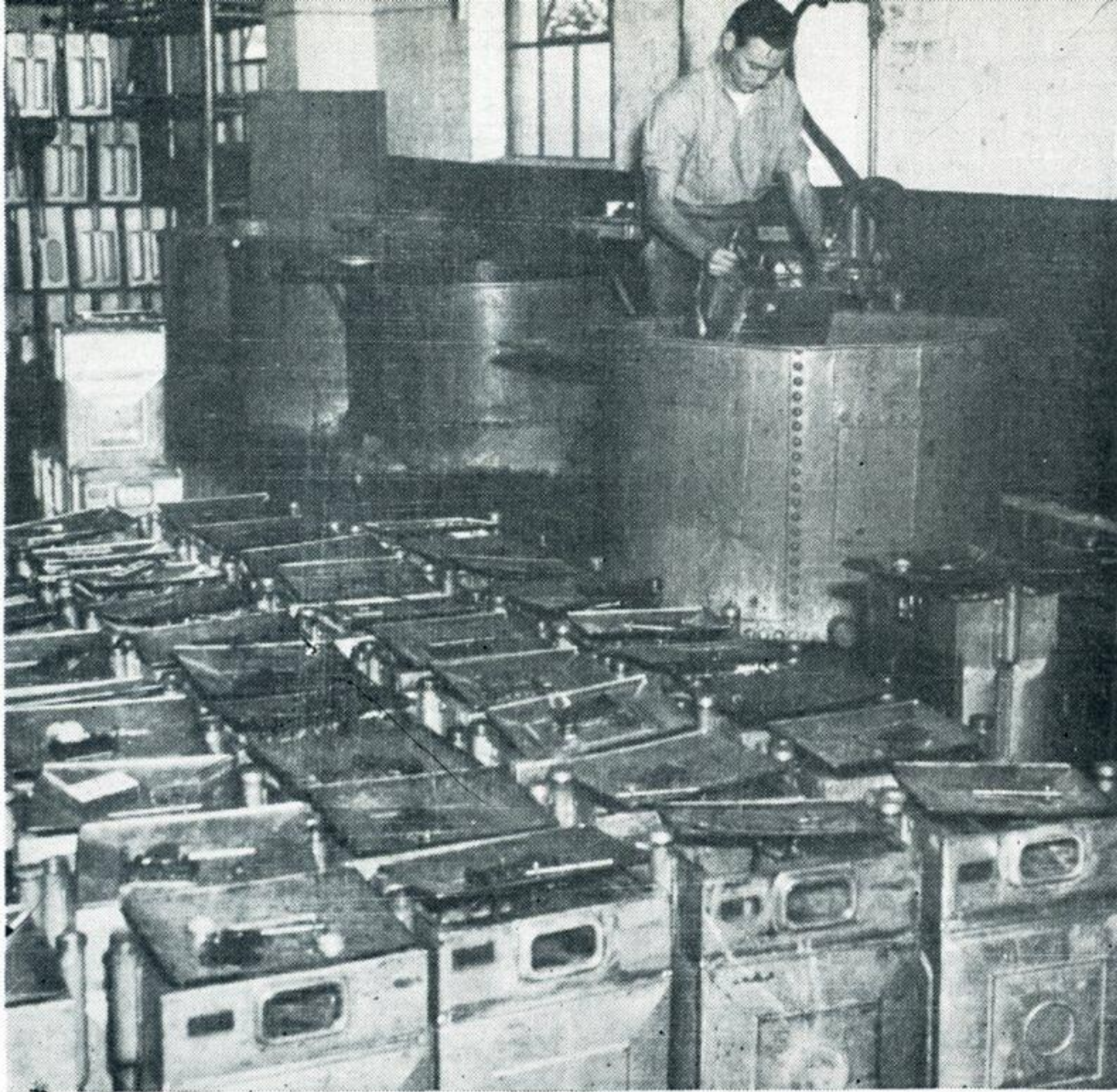
THE GAS DEPARTMENT spent most of the summer repairing meters for winter. Shown on these two pages are some typical preparatory activities. At left John Greer runs air through a meter box and inserts it into the cylinder filled with water to test it for air leaks. Above are Albert Weimer, John Greer, Mark Couvillion and Allen Carpenter soldering meter boxes. Bill Humphries is pushing the dolly full of meters.
