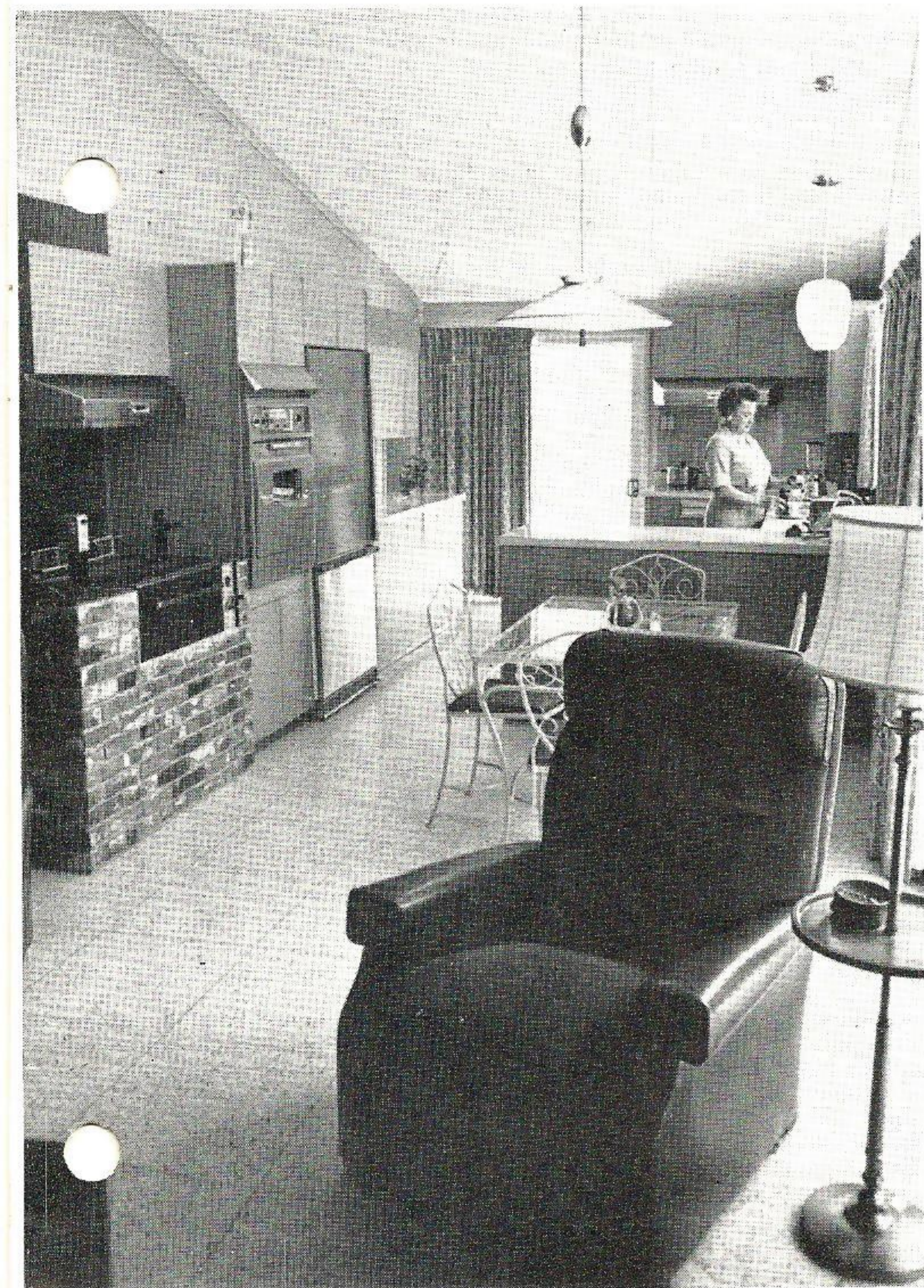
THE ALL-ELECTRIC KITCHEN. The handsome built-in oven, refrigerator and table top range are of matching hues of rusk. At left is a charcoal grill made of old fashioned brick over which hangs a stainless steel spit for barbecuing and charcoaling. The Nutone hood over rotisserie is vented through roof to keep charcoal fumes out. Pull-down lighting fixtures illuminate the room. Serving bar has cabinets that open on both sides for ease in obtaining dishes.
