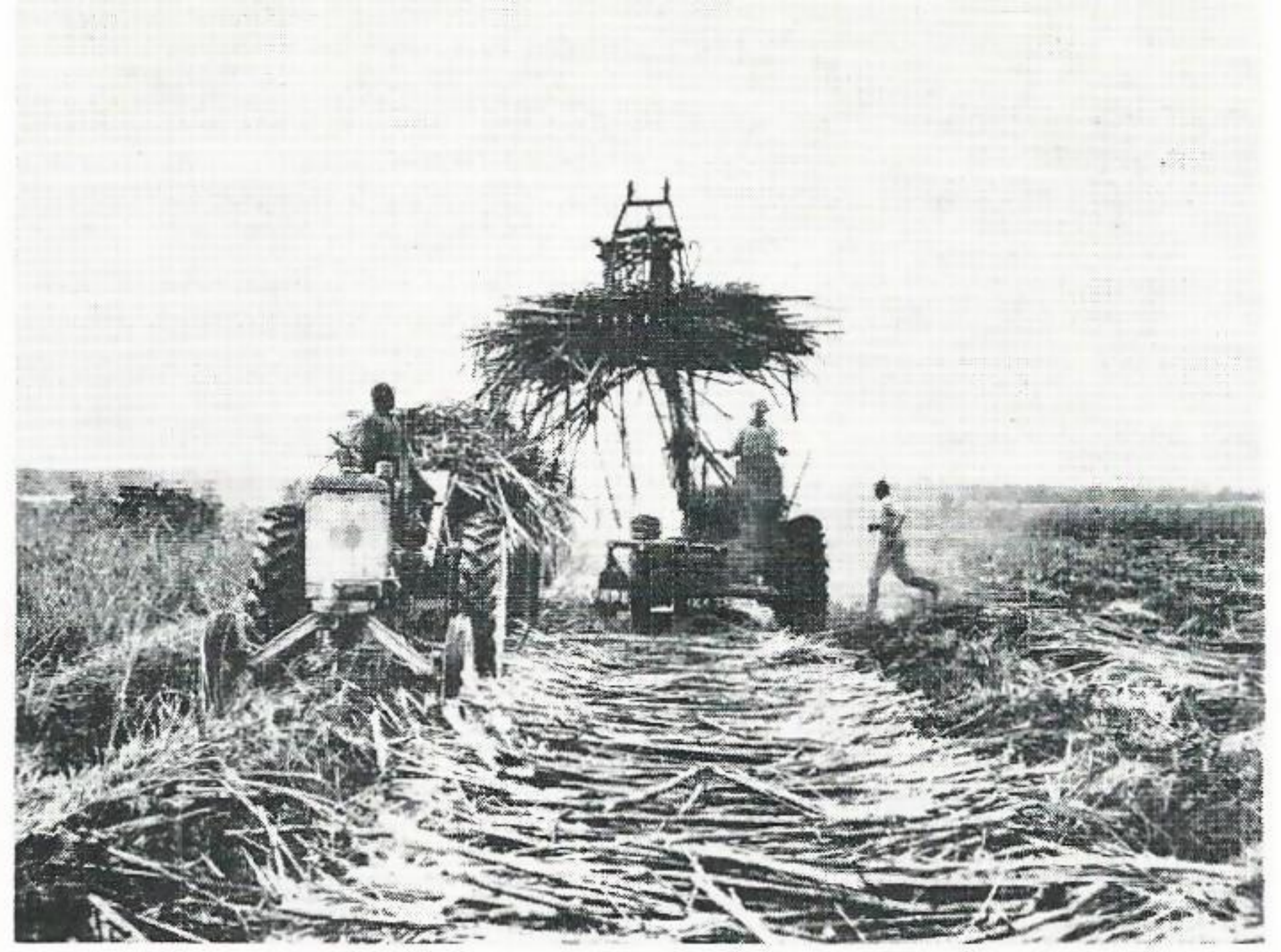
LOADING. The Thomson Machinery Co. of New Orleans introduced the first sugar cane harvester in the 1930's. The same company devised the "Hurricane" loader which gathers and loads the cane into waiting cane wagons in one movement.
