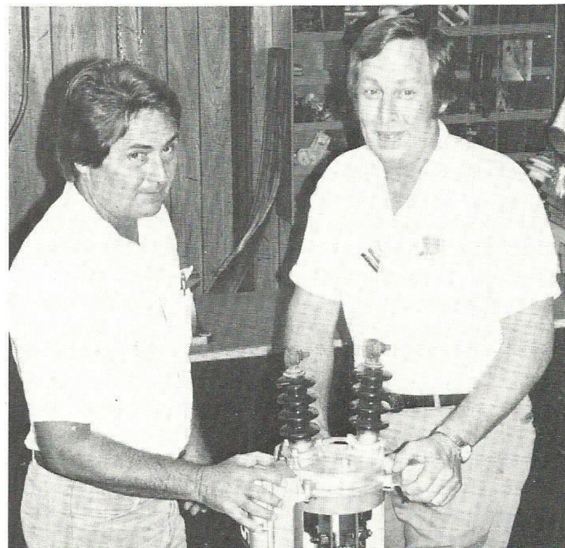
Jack Winston, mechanic-1st class of Baton Rouge, shows Steve Moore of Port Arthur (middle) and Jed Gerbrecht of Baton Rouge (left) how to install a "cat head" on a line truck. The equipment will have rope wrapped around it and then be used for dragging heavy items.
