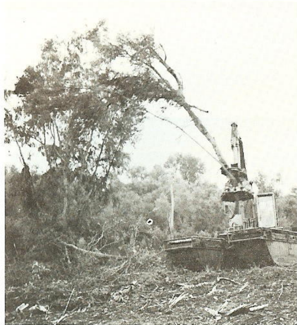
A tree-chewing tractor clears the right-of-way (above) before beginning the float to the next island (right). GSUer Mike Laborde checks progress with one of the contractors clearing for 500kv Line 760 (below).
